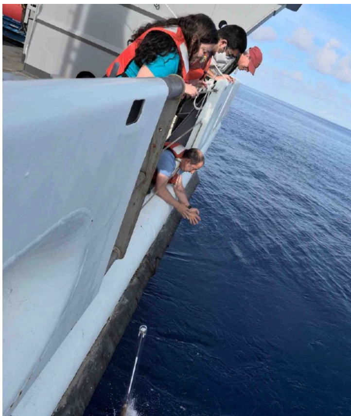
RAFOS float deployment. These floats are ballasted to 4000 m. The deployment during the A22 is at-sea test for the Deep Madagascar Basin Experiment next year. Observe our flat sea. Photo: Mike Wazowski
