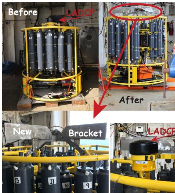
Figure 1: Before (upper right) and after (upper left) views of the rosette illustrating the newly designed bracket (lower left panel) and its position protecting the rosette instrumentation as it docks with CAST-6 (lower right panel).
