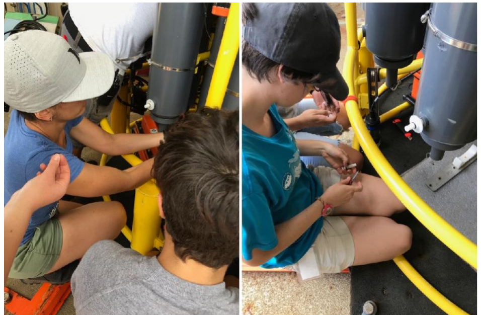
Figure 4: CTD-watch learning about the rosette from ODF guru John Calderwood, in the midst of replacing 108 O-rings. Photo credit: Alison Macdonald
